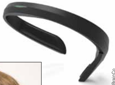
Photo 1 (above)—The Focus1 BMI captures brain-waves from its contact points on a person's skull
