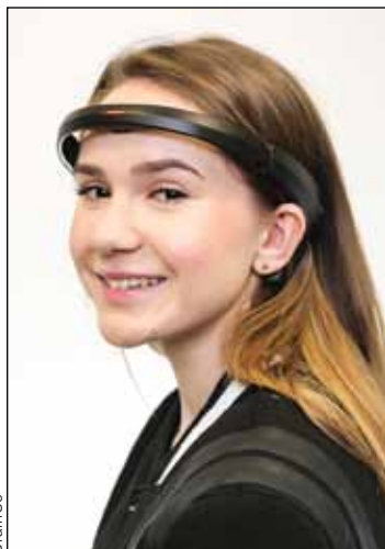
Photo 2—The BrainCo BMI uses electroencephalogram (EEG) technology, but with much fewer contact points on a person's skull than a medical EEG.
