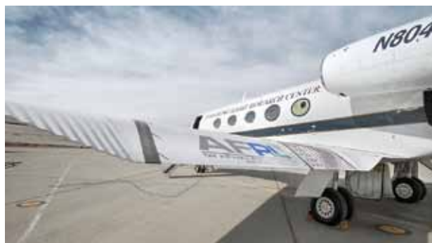
Photo 1—NASA used this Gulfstream airplane to flight test the ACTE morphing wing technology.
