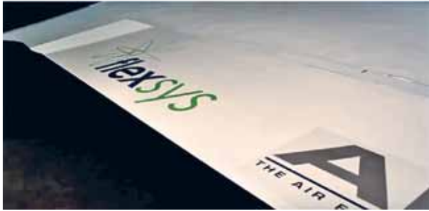
Photos 2 and 3—The morphing flap lies perfectly flat (left) until it needs to be adjusted. It can morph its shape from 2° up to 30° (right) and hold its shape at any degree angle requested by the pilot.
