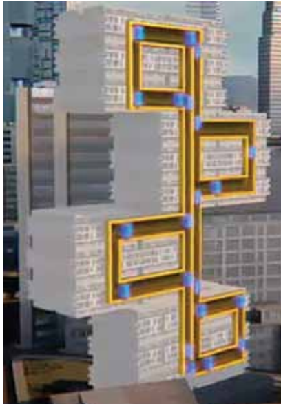
Fig. 4—The ThyssenKrupp vision calls for MULTI to develop into a vertical and horizontal transportation system.
