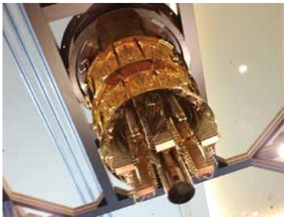
Photo 1—For this quantum computer to operate properly it must be cooled down to almost absolute zero.
