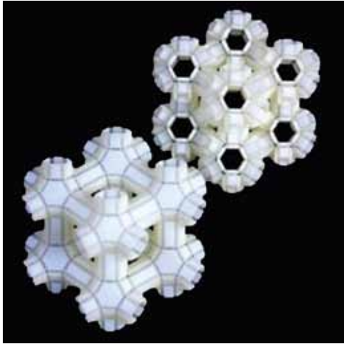
Photo 5—The two metamaterial objects in this photo look different but they are the same object. They were created using the new Harvard technology so they can shape shift. By building in this ability this metamaterial can shift its functional properties.
